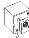
外径φ4、内径φ2.5のチューブなど Example of a tube with external diameter of φ4 and internal diameter of φ2.5
